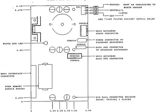
Note: Card is not drawn full scale. See DIN RAIL RELEASE DETAIL page 4.
